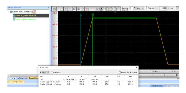
When using "MC\_MoveRelative" function, the Distance is 600mm, the Velocity is 60mm/s, the Acceleration and decleration is 60mm/s^2.
